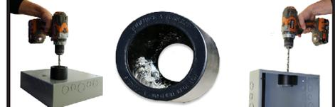
Clamp to bottom or top of metal surface using rare earth magnets to catch metal shavings
